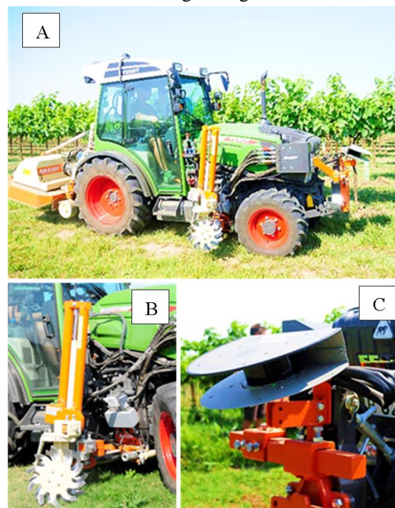
Fig. 2. Working configuration (A) with tillage implement (B) and sensor (C)
